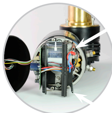
Threaded rods for motor outer cover attachment screws
