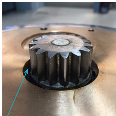
Lubrication of motor drive shaft lip seal.
