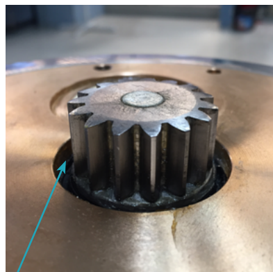
Lubrication of motor drive shaft lip seal.
