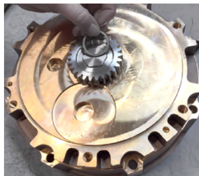
Remove the circlip to lift the drive gear and expose the lip seal in the shaft recess.
