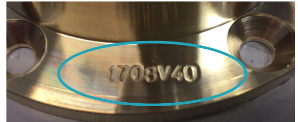
Winch production year and month [YY-MM] followed by version number are stamped on winch base between the mounting bolt holes.
