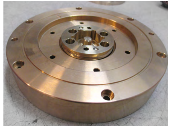
Gearbox in position, ball race ready for loading
