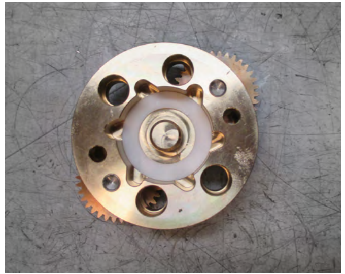
Planetary drive gear unit removed
