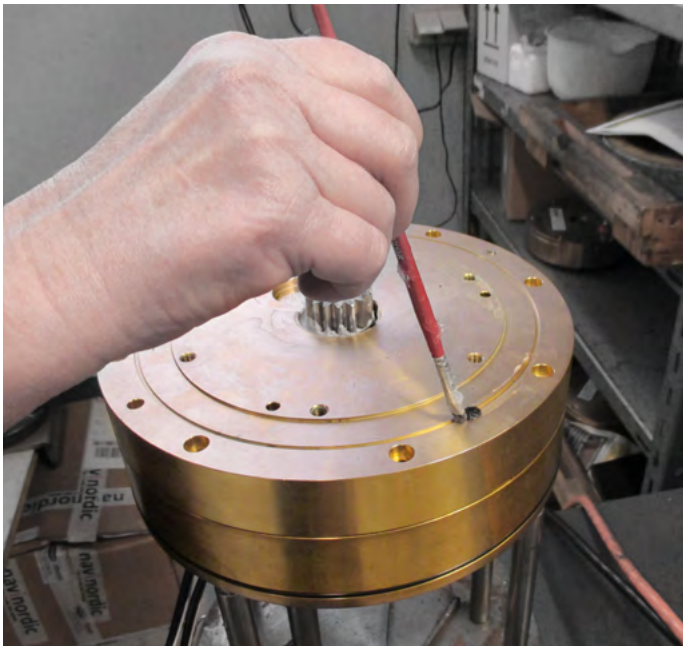
Apply Andersen Winch Grease to O-ring recess
