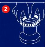
Stretch over top of winch with ribs facing downwards.
