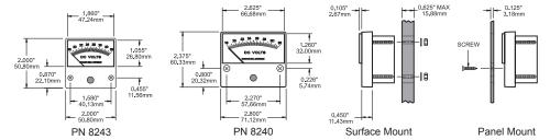
Surface Mount: Drill five clearance holes as shown below. The part number of the meter will determine the size and location of the clearance holes. Use the nuts and washers supplied in the accessory package to secure the four mounting studs to the mounting surface. This method will work on mounting surfaces up to 5/8" thick.
