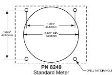
**Panel Mount:** For thicker mounting surfaces, the meter can be mounted into a 0.125" thick panel. Blue Sea Systems offers meter mounting panels for our standard size meters only. For PN 8240 use PN 8013 to mount a single meter or PN 8014 to mount two meters.
