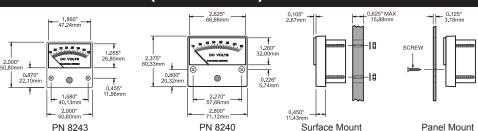
Surface Mount: Drill five clearance holes as shown below. The part number of the meter will determine the size and location of the clearance holes. Use the nuts and washers supplied in the accessory package to secure the four mounting studs to the mounting surface. This method will work on mounting surfaces up to 5/8" thick.
