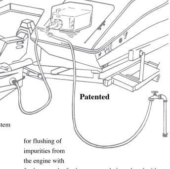
fresh water, the fresh water supply is replaced with antifreeze to winterize the engine for storage. For additional insurance the thermostat may be removed. Thermostat removal is not necessary if the following step-by-step instructions are followed explicitly.
