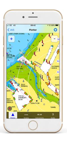
Our iAIS app is now available with a Navionics plug in allowing AIS targets to be overlaid on a Navionics chart layer
