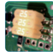
Easily accessible fuses
