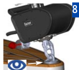
3 Check the positioning of the snapshackle in the chainplate
