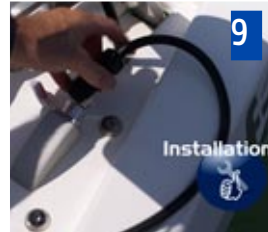
4 Plug the drive unit onto the deck socket
