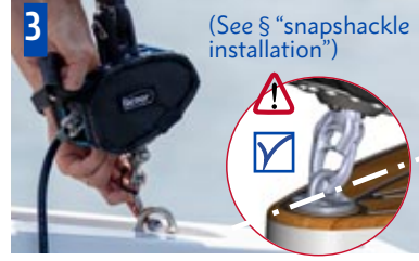
3 Check the positioning of the snapshackle in the chainplate
