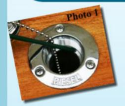
Begin by examining your deck fill to determine if the area below the threads has a narrowing ridge as in Photo 1 or is ridgeless as in Photo2.
