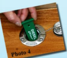
If deck fill is Ridged, simply insert the appropriate FillGuard into the fill. If the "T" bar is too wide, snip a little off each side until it fits loosely atop the ridge. Use the scribed guide lines on top as a reference. Cut with a garden snips or sharp wire cutter (see Photo 3). Proper fit is achieved when FillGuard is easily removed with two fingers (see Photo 4).
