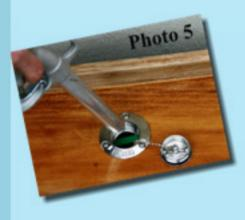
If deck fill is Ridgeless, use the enclosed stainless ball chain and bail fitting. Cut FillGuard's top "T" bar close to the base with garden snips or some sharp cutter. Remove the deck fill cap's safety chain retaining screw and reattach with the provided bail fitting. Use super glue or Loctite on screw threads to prevent screw from loosening. Do not glue the bail fittings. When replacing the screw be sure not to over tighten.
