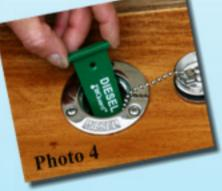
Once in place, FillGuard prevents inserting the filling nozzle until removed, thereby causing the user to confirm the correct fill has been selected (see Photo 5).
