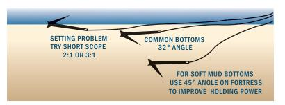
The Fortress flukes can be adjusted from the normal 32 degree angle to 45 degrees to increase holding power in soft mud bottoms by as much as 400%. Also, special "Mud Palms" are included for both Fortress and Guardian anchors to aid setting in very soft problem mud. We recommend that you permanently install the "Mud Palms" on your anchor, as they will help the anchor set faster in any type of bottom.
