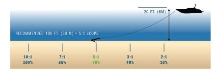
At less than a 3:1 scope, you will give up a significant amount of holding power and may experience problems setting the anchor.
