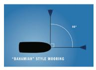
Any anchor can fail to reset once it has been pulled out of the sea bottom. Don't be fooled by some manufacturer's claims about an anchor's ability to dependably reset 100% of the time. Set two anchors if you expect a change in current or wind.
