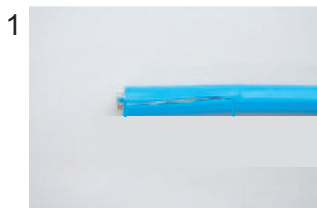
1 Expose inner vinyl sheath.
