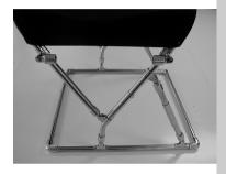
Tension the frame using straps, line etc. Position the 4 sliding side mounts as desired. They will usually be parallel to the fabric edge. Secure them using the set-screws. Install an eye end on each side mount. Position them to face each other as shown. Photo 2
