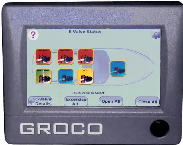
LCD-5 touch screen allows monitoring and control of all E-Valves on your boat. The screen is water resistant and can be flush mounted (4-3/8" high x 4-1/2" wide) or bracket mounted (bracket included).
