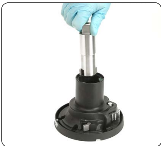
8. Slide out the central shaft n°7
