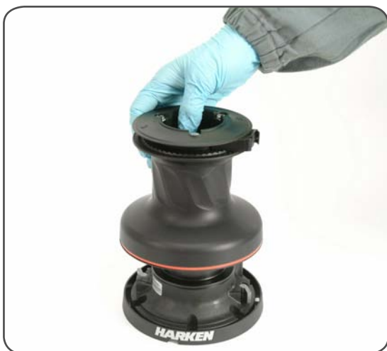
5. Lift off the drum n°13
