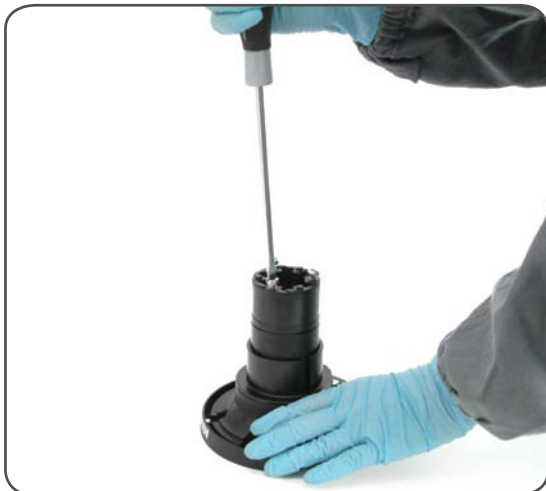
6. Completely unscrew the three screws n°17
