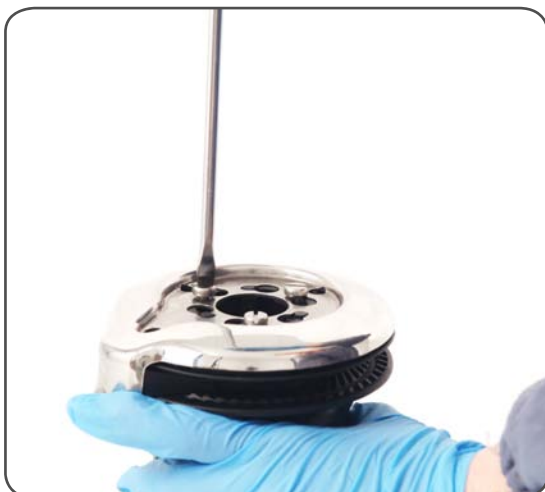
3. Unscrew the three screws n°17 ( \approx 4\text{Nm}/35\text{ in-lb} )
