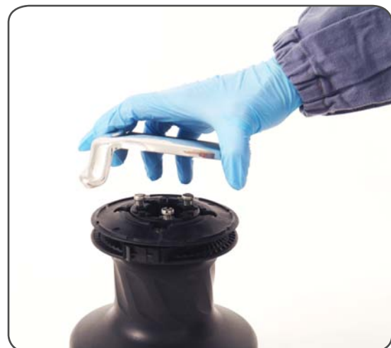
4. Remove the self-tailing arm n°18 by rotating and lifting it.
