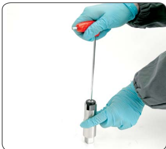
Unscrew the screw n°10 and remove the washer n°9 ( \approx 4Nm/35 in-lb)
