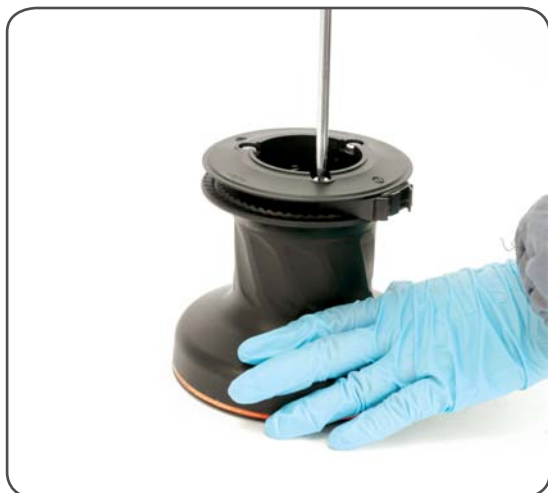
I. Unscrew the 3 screws n°16 ( \approx 4Nm/35 in-lb)
