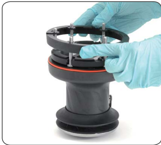
4. Reposition the skirt n°2 in its housing
