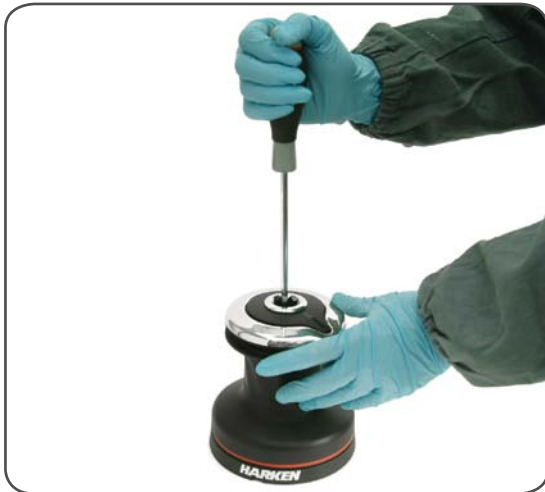
1. Unscrew the central screw ( \approx 2\text{Nm}/18\text{ in-lb} )
