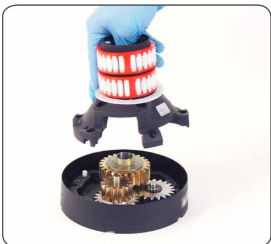
10. Remove the drum support n°15 Important: washer n°12 may remain inside the drum support!
