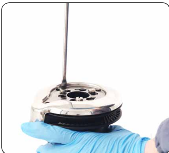
3. Unscrew the three screws n°27 ( \curvearrowright 4Nm/35 in-lb)
