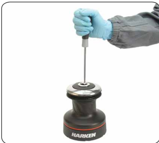
1. Unscrew the central screw ( \curvearrowright 2Nm/18 in-lb)
