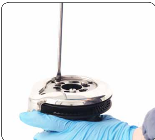
3. Unscrew the three screws n°29 ( \approx 4\text{Nm}/35\text{ in-lb} )
