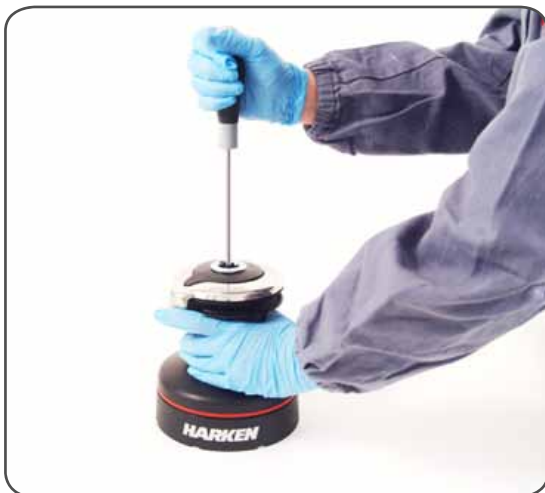
1. Unscrew the central screw ( \approx 2\text{Nm}/18\text{ in-lb} )
