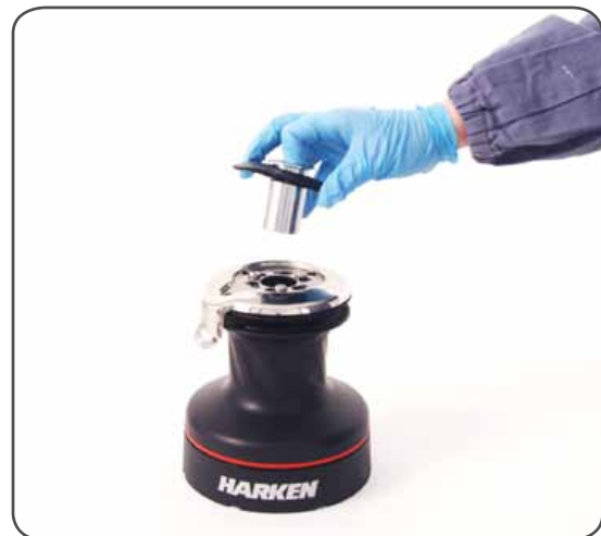
2. Slide off the assy socket n°31 and the cover n°30
