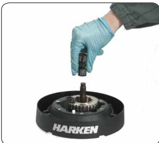
15. Remove roller bearings n°12 and spacers n°13
