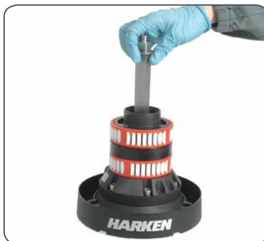
7. Slide out the central shaft n°21
