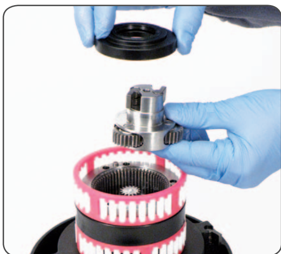
9. Remove the second planetary assy n°24 and remove flange n°11. Pay attention to the o-ring in the ring gear.
