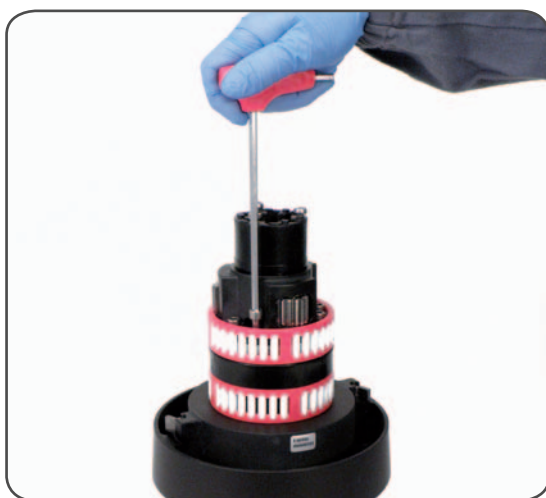
5. Unscrew the 5 hex screws n°18 (20Nm/177 in-lb)
