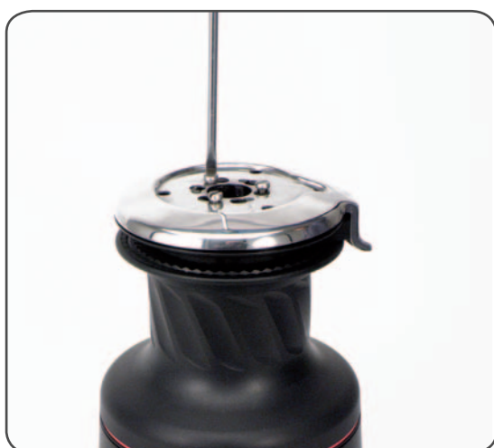
3. Unscrew the three screws n°25 ( 4\text{Nm}/35\text{ in-lb} ) and remove the self-tailing arm n°8 by rotating and lifting it.
