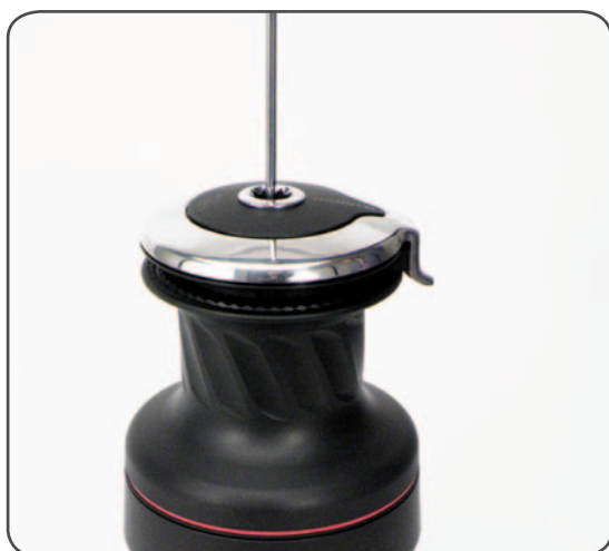
1. Unscrew the central screw ( \approx 2\text{Nm}/18\text{ in-lb} )
