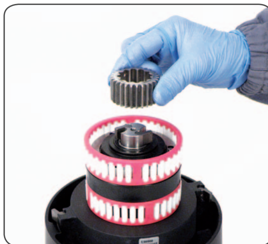
8. Lift off the gear n°9
