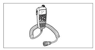
The optional HM-195 should be connected to the transceiver using the supplied OPC-1540 connection cable.
