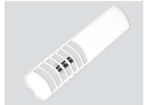
A dedicated air temperature sensor continuously measures cabinet air temperature. This sensor replaces the mechanical probe fixed to the evaporator on your old system.
