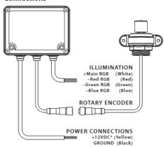
\* Install a fuse at the +12VDC Power Wire (Yellow) connection point that is appropriate for the total current draw of all LED circuits.
