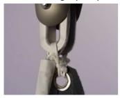
\*If the thimbles being used are not the ones supplied by Karver, they must use the maximum width of the fork. If this is not the case, a bending load will be applied to the pin and its mechanical resistance will be weakened. Karver cannot guarantee the safe working loads if other thimbles are used.
