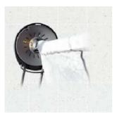
• Pull on the left line of the continuous line to furl (a marking "Furl" scribed on the spool indicates which side of the line to pull on). If the furling line is accidently released, the mechanism will lock automatically.
