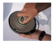
• To remove the lock, pull on the conical piston and slide it out of the drum. The unit will now work in either direction. To remove the lock, pull back on the conical piston and slide it out of the drum. The unit will now turn in both directions.
