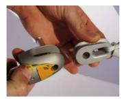
• Push the pin completely back in to lock the thimble in place.
