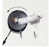
• When the sail is entirely furled, release the continuous line and the drum will automatically lock.
