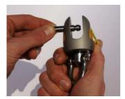
• Install the tack thimble into the drum fork and the head thimble into the top swivel fork.
