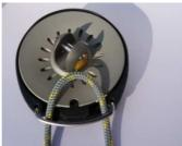
• Fit the line into the notch of the wheel on the right of the ejector.
