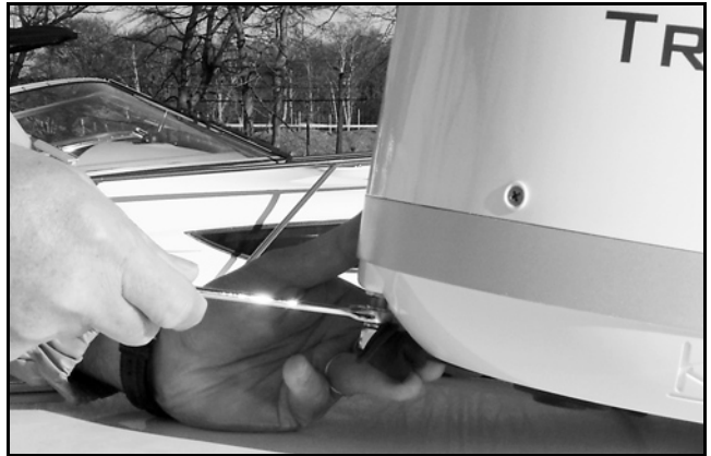
Figure 11: Connecting the Antenna Cable
