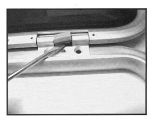
Adjustment of the hinges is made by turning the jacking nut and bolt (see photo) with two small pins eg small hexagon key. Holding one part still and rotating the other anti-clockwise will increase the friction. Adjust each hinge by 1/4 a turn at a time and check the adjustment.
