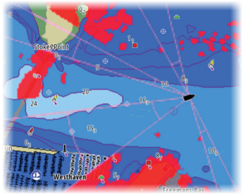
Radar overlay on a chart
