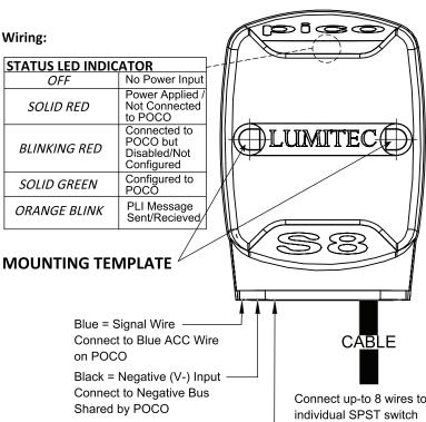
Red = Positive (V+) Input – Connect to 10-30VDC Power Source. FUSE APPROPRIATELY Connect up-to 8 wires to individual SPST switch outputs. *Optional*: Connect to switch's indicator LED
