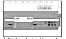
1. Slide Grease Tray into either side of the mounting bracket to lock.
