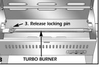
**3.** To remove burner pull locking pin.
