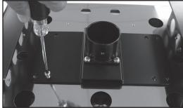
2. Locate (8) threaded inserts on bottom of firebox. Using (8) 1/4-20 x 3/4" pan head screws and Phillips head screwdriver, install adaptor plate to firebox.
