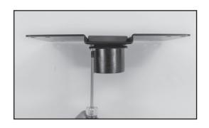
1. Using supplied (4)  $\frac{1}{4}$ -20 x  $\frac{1}{2}$ " pan head screws, (4)  $\frac{1}{4}$  washers (supplied with pedestal mount assembly) and Phillips head screwdriver, install pedestal top cap and pedestal adaptor plate to grey aluminum mounting pad. Ensure flat side of pad is at top of assembly with hollow side facing down towards bracket and top cap.
