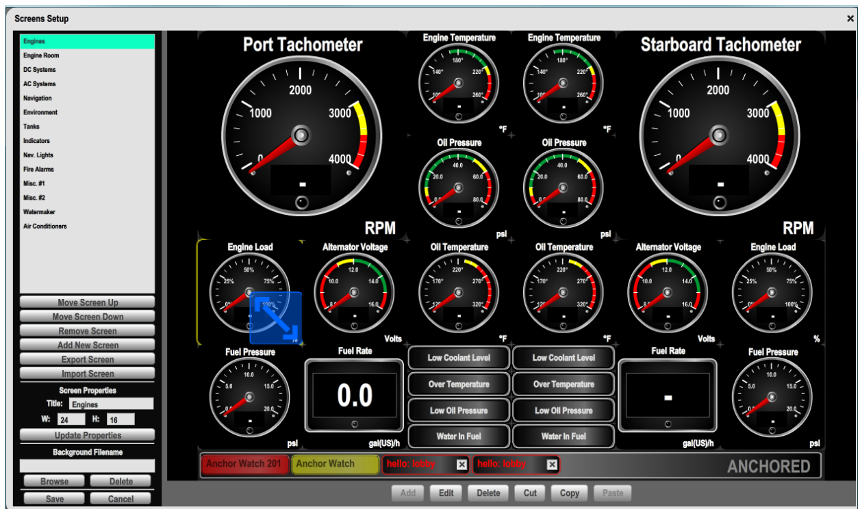
Figure 23 – Screens Setup Screen
