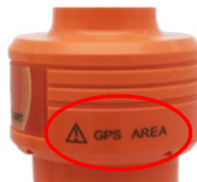
Figure 6: GPS/GNSS AREA Location
