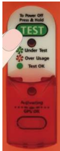
Figure 11: Testing of AIS SART
