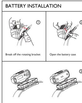
According to the correct polarity to join AA batteries
