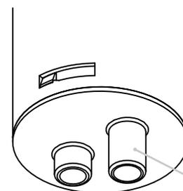
Drain hose connector  $\varnothing 14$
