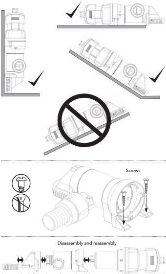
Best practice: Periodically clean the sensor housing with a mild detergent to remove any build-up that may interfere with the proper operation of the bilge pump. If the sensor accumulates excessive build-up, the pump will enter the timer mode to protect the pump and the vessels batteries. Once the debris is removed, the pump will return to level sense mode.
