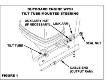
Thoroughly clean the inside of the tilt tube and regrease using a waterprooof marine grease.
