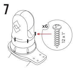
Secure the adapter to the ADA-F2 top plate using the provided six #12 x 1" screws with a philips head screwdriver.
