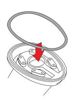
Insert rubber gasket onto the top of the Seaview mount. (Rubber gasket included with Seaview Mount.)
