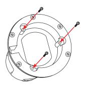
Secure the FLIR M100 or M200 to the adapter with the hardware specified by your electronics manufacturer.
