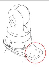
The four holes on the back of the ADA-F2 are for securing the optional Seaview Light Bar to the top plate..
