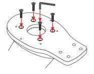
Secure the ADA-F2 with the four bolts using an allen 3/16" wrench.
