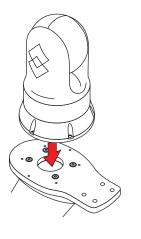
Plate the FLIR camera ontop of the ADA-F2 top plate. Make sure that the six holes on the adapter line up with the six holes on the top plate.
