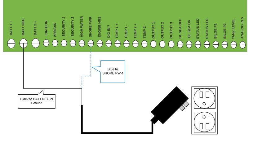
To use the MTC to monitor connection to Shore Power, either the Siren Marine Shore Power Sensor Plug or an AC Relay are needed.
