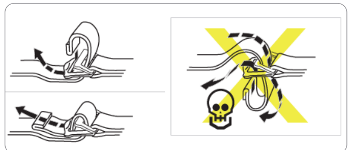
Correct threading of Deckvest 6D adjustment straps
