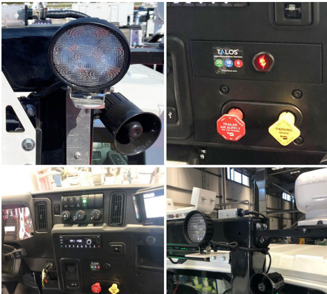
Remote Lightning Detector with Horn Installation
