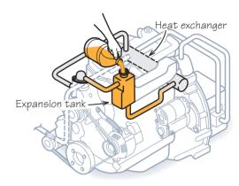
Fill system with a pre-mixed solution of water and TRAC Descaler Concentrate<sup>®</sup> (see product label for correct dilution ratio).
