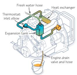
Drain solution and flush system until all traces of the TRAC Descaler® solution are removed.
