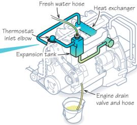
Drain coolant from engine and flush with fresh water to ensure all the coolant has been completely removed.
