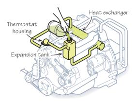
Secure drain valve, replace thermostat and fill the engine with engine coolant (see manufacturer's specifications).
