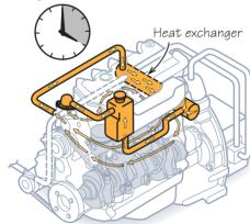
4 Start engine to circulate solution through internal cooling channels. Run engine intermittently on and off every 30 minutes for four hours.
