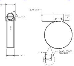
Premium Marine Grade, all AISI 316 (high tensile strength) Stainless Steel "HD NON-PERF" Worm Gear Hose Clamp. The 11.7 mm (0.46") wide band is Non-Perforated and Smooth on the inside with Rolled Edges. This eliminates hose damage with increased clamping force. The High Strength, Compact, One Piece 16mm (0.63") wide Housing provides one of the highest clamping force ratings of any worm gear style clamp. Screw Head is 7mm.
