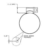
Premium Marine Grade, all AISI 316 (high tensile strength) Stainless Steel Compact "HD NON-PERF" Worm Gear Hose Clamp. The 9.7 mm (0.382") wide band is Non-Perforated and Smooth on the inside with Rolled Edges. This eliminates hose damage with increased clamping force. The High Strength, Compact, One Piece 14mm (0.55") wide Housing provides one of the highest clamping force ratings of any worm gear style clamp. Screw Head is 7mm.
