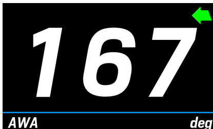
Layout MAST : four pages with data about: A pparent wind angle ( AWA ), A pparent wind speed ( AWS ), S peed through water ( STW ), T rue heading.
