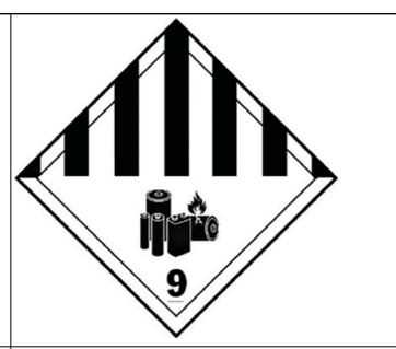
The additional following placard must also be placed visibly in proportion to crate size but must be no less than 120x110mm.
